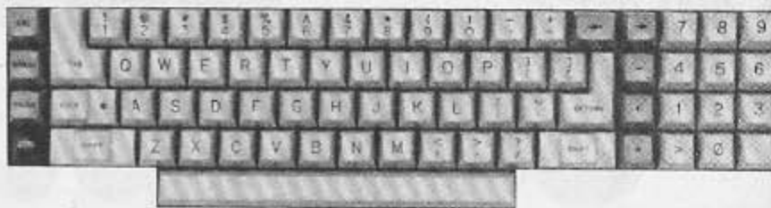
The Franklin ACE 1000 keyboard includes a 12-key numeric pad, an alpha lock key and keys with special VisiCalc designations.
